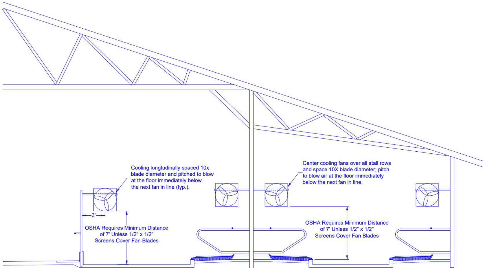
Figure 1. Lateral positioning of cooling fans over feeding cows and lying cows in a freestall barn.
