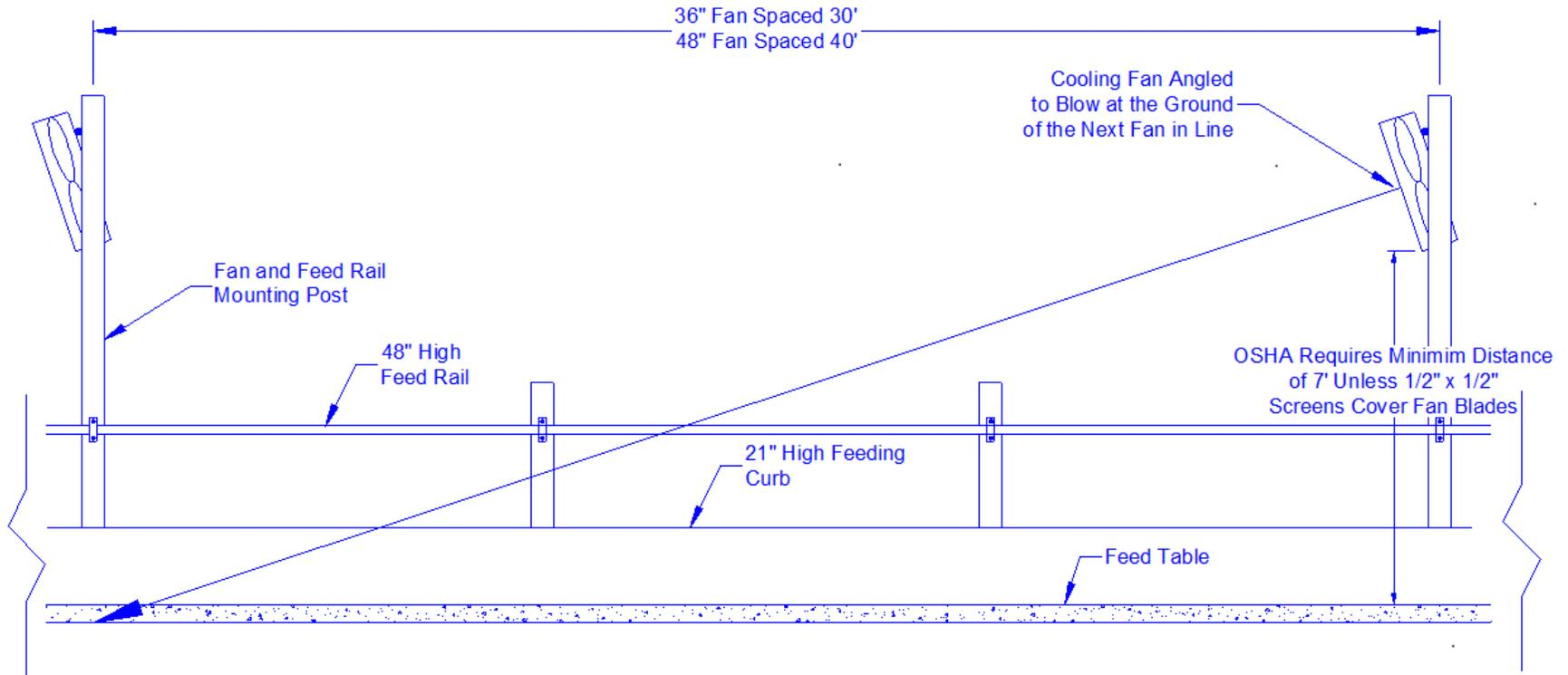
Figure 2. Longitudinal positioning of cooling fans over feeding cows in a freestall barn.
